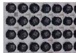
Rack base : 2D Datamatrix barcode under each tube and the rack
