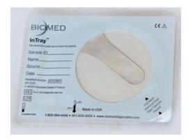
The patented InTray™ system consists of a reclosable outer seal containing an optically clear, antifog window. The seal creates an airtight 2" diameter chamber providing a large enough area to streak for isolation. The innovative design of the InTray™ high-performance viewing window makes it possible to place the device directly under a microscope. This removes the need to prepare slides and prevents unnecessary exposure of the sample after inoculation.
